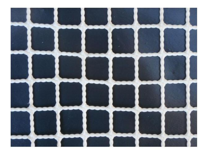
K-Grid netting technology is made of a high tenacity knotless resin treated weave that is heat treated providing a smooth strong surface. These nets provide advanced predator exclusion measures.
